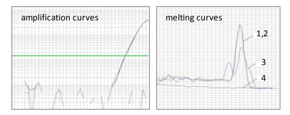
**Figure 1.** Highly specific amplification with Arraystar Master Mix. In the postamplification melting curve analysis, the PCR products by Arraystar Master Mix had single peak dissociation profiles (1 and 2), whereas the PCR products by master mix from competitor A (3 and 4) produced multiple dissociation peaks.
